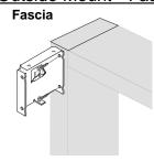
The roller brackets can be mounted back against the window casing, or up against the ceilina.
