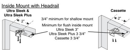
Use shims if necessary to ensure that the headrail is mounted level (included).
