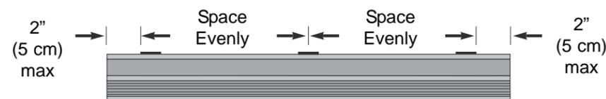
Depending on the width of the shade, additional brackets may be necessary and should be evenly spaced between the two end brackets.
