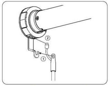
On Banded Shades, Roller Shades and Sheer Shadings, with the wand control buttons facing you, attach the top of the wand on the metal hook support (1) on the motor control side, then connect the cable into the motor head (2).
