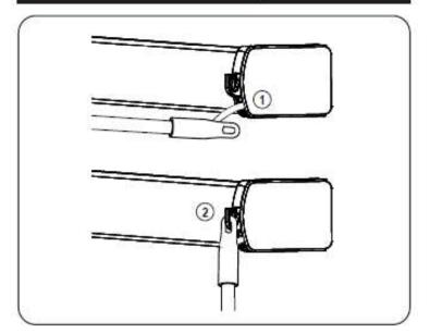
On Honeycomb shades, the wand will be already connected to the shade (1). With the wand control buttons facing you, attach the top of the wand into the plastic hook support on the motor control side (2).
