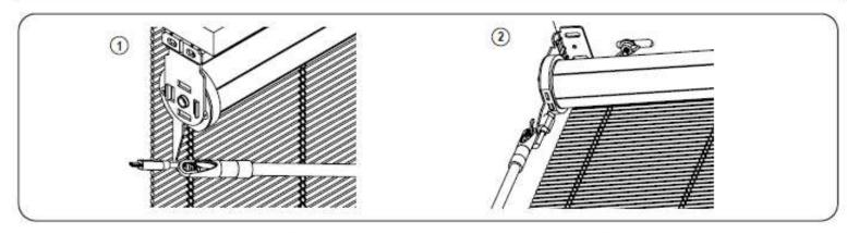
On Natural Woven Shades, with the wand control buttons facing you (1) approach the hook with the wand parallel to the headrail. (2) Gently twist the wand to attach it to the hook. Connect the cable into the motor.
