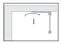
Align screw through the front hole of the Inside Mount Bracket and the center groove of the Valance.
