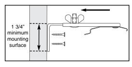
Set the bracket to the smallest position, so that the standard valance returns will fit properly. Position the mounting bracket at the desired height. Place a screw through the center of the slotted hole on the mounting bracket and secure into the mounting surface. Make sure that all mounting brackets are level. Secure brackets with a second screw through the round hole.
