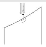
Push the louver up into the carrier stem, then pull slightly straight down to lock into place.
