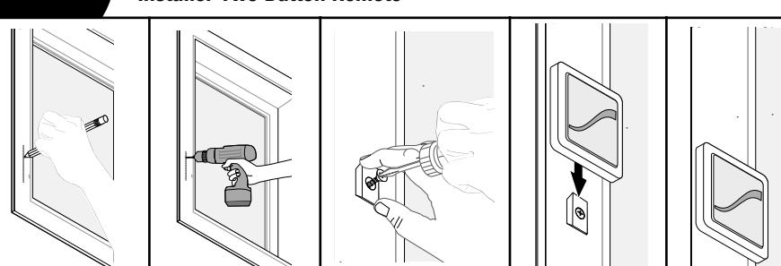
Mark screw location. Drill hole. Screw into place. Slide Two Button Remote into place.
