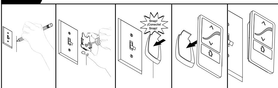
Mark screw location. Drill hole. Screw into place. Snap bracket into mount. Insert Single Channel Remote.
