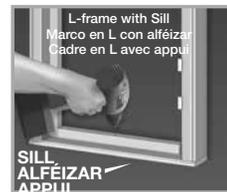
While frame is still on the floor, use a 1/8" drill bit to pre-drill one hole on each side of the frame approximately 3" down from the top of the frame (see picture). Pre-drill one hold in the center position of the bottom frame, or as close to the center as possible if you have a T-post in your frame. If your frame has a bottom sill frame piece, pre-drill the bottom hole as shown above right.
