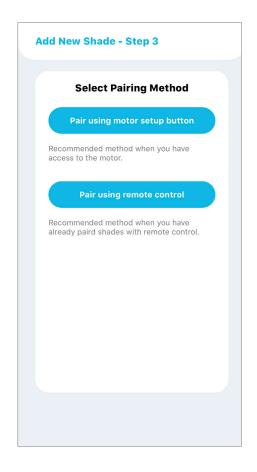
AMP Tip: When using the "Pair using motor setup button" method, you will need access to the setup button (P1 button) located on the motor.
