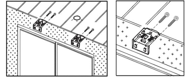
Make sure brackets are aligned. "L" shape opening should be facing down, with shorter side against the wall.
