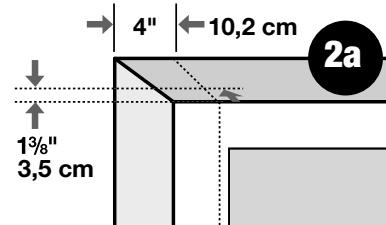
Hold headrail up, centered over the door or window. Measure 4" from each end. Space additional brackets evenly along the headrail. Mark bracket locations **at least 1<sup>1</sup>/<sub>8</sub>" from window.**
