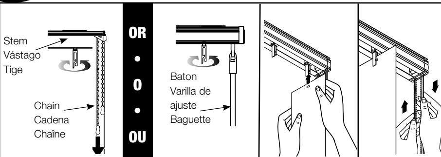
To realign stems, rotate louvers fully in both directions.
