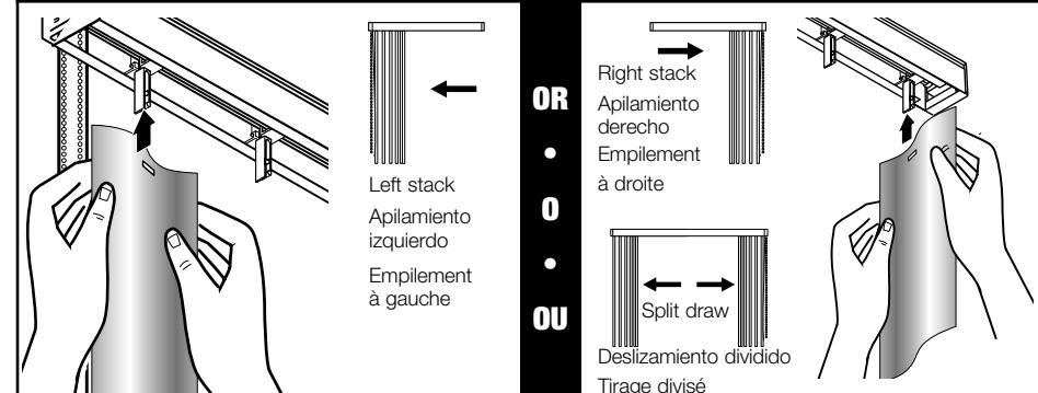
**Vinyl S-shaped Louvers:** S-shaped louvers are NOT reversible. On right stack & split draw, the high side of the louver is to the right of the louver stem hole. On left stack only, the high side of the louver is on the left side of the louver stem hole.
