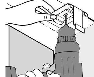
Drill holes marked for bracket locations. Note: For louver clearance, the mounting clip must line up with the marking for flush louver mount (Step 2c).
