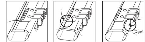
For style 'B' [see illustration below]: Lift the Head Rail into position such that the front edge of the bracket is under the inner front edge of the head rail, and then push the head rail upward until the flexible tab at the bottom of each bracket snaps onto the back of the head rail. Check carefully to assure that each bracket is properly secured.
