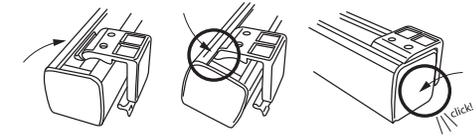
For style 'C' [see illustration below]: To attach the brackets the locking arm should be facing out. Then position the bracket so that it engages the inner front and outer back of the head rail, and then push the locking arm inward to lock it in place.
