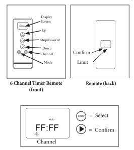
Use the **STOP** button to select the day and move on to the next one. Use the **UP** arrow to skip a day and the **DOWN** arrow to back up. You must press **STOP** for each day that you want to select. If the day is still flashing, it has not been selected.
