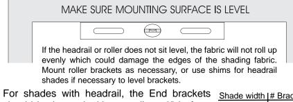
should be located with centerlines 2" in fr each end. Depending on the width of shading, necessary additional brackets m be evenly spaced between the two e brackets.
