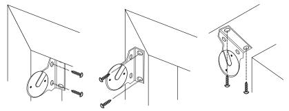
Mark the screw locations with a pencil - pre-drill the screw holes using a 5/64" drill bit.
