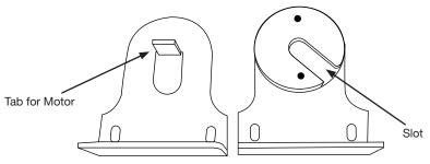
Note that the bracket for the motor end of the shade has a tab that fits into the motor housing. The Pin-End Bracket has a slot that the pin end slides into.
