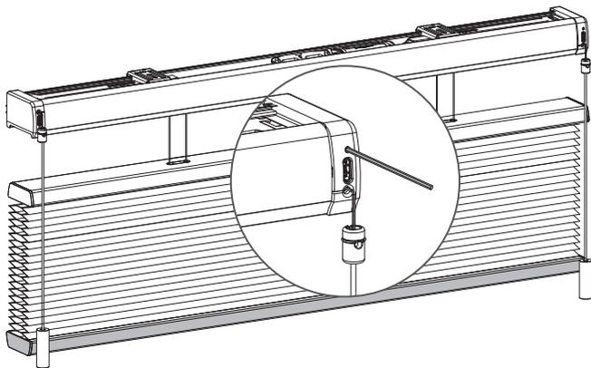
1 Pair the bottom rail motor to an empty channel on the remote. (see step 1)
