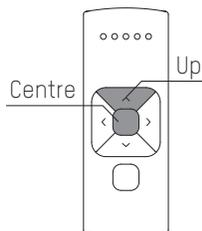
2 Check the direction of rotation of the bottom rail (see step 2) and move the bottom rail to the desired top position. Simultaneously hold the centre and the down button on the remote until the blind stops stepping and starts stepping again. The top position has been saved
