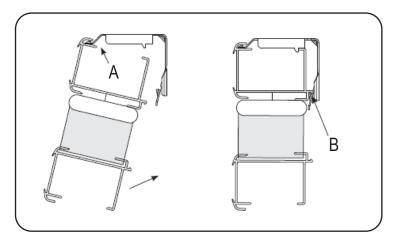
Start with the top rail (the rail with the motor in it). Make sure that the receiver wire is out of the headrail before mounting. Position the receiver wire so that it is facing into the room and position the motor wire so that it comes out the back side of the shade, ensuring it is not pinched by the bracket.
