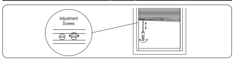
If the moving rail is uneven it can be leveled using the shade adjust on the bottom of the rail. Use a flat head screwdriver or a dime to turn the adjustment screw to raise or lower that side of the bottom rail. The adjustment screw is on the bottom of the moving rail. One quarter turn of the screw will move the moving rail up or down approximately 1/4"
