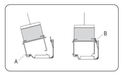
Position the rail with the front lip (A) resting on the hooks of all the brackets. Push the rail firmly down and toward the window until the groove on the rail snaps into place, (B) as shown.
