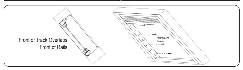
Place the track against the front of the top and bottom rails. Attach the track with the screws provided. Space the screws no more than 12" apart. Follow the same procedure for the other track. Make sure that the 2 tracks are parallel to each other.
