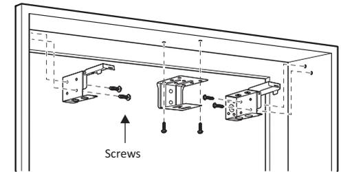
If Center support Brackets are included, evenly space them between the two end brackets. Be sure they are positioned in a way they do not interfere with the blind operation.
