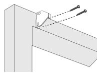
The roller brackets can be mounted back, against the window casing, or up, against the ceiling as pictured for Inside mount.
