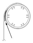
Roll the shade up and check for skewing. If the shade is still skewing, add another strip of tape on top of the first one. If the shade is now skewing to the opposite direction, tear off about 1" of tape from the last strip installed. The tape is to be torn from the end closest to the center of the shade.
