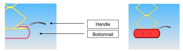
3. If installing a second handle on a cordless top down/bottom up shade, insert front lip of bottomrail handle onto the bottomside of the middlerail. Handle will be reversed orientation of the bottomrail handle with the brand facing downward. Handle will snap into place.
