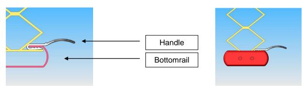
6. If installing a second handle on a cordless top down/bottom up shade, insert front lip of bottomrail handle onto the bottomside of the middlerail. Handle will be reversed orientation of the bottomrail handle with the brand facing downward. Handle will snap into place.
